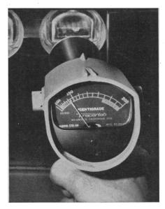
Pyrometer shows that Tracerlab's LTA-600 can ash samples thoroughly at temperatures well below 150°C—low enough to leave all inorganic constituents unaltered. A cold plasma of atomic oxygen does the ashing, while our accessory pyrometer keeps you posted on the temperature.
