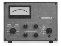
ESI has combined the best features of the classic galvanometer and the modern electronic voltmeter in the Model 900 Nanovolt Galvanometer.
