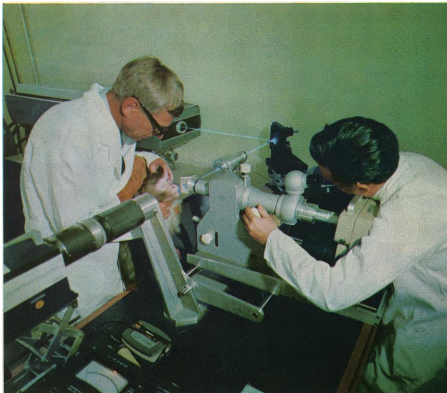
In initial tests using a rhesus monkey, two members of the research team at Stanford control the blue-green beam from a Model 140 continuous wave argon laser by means of a shutter mechanism and an optics aiming device.
