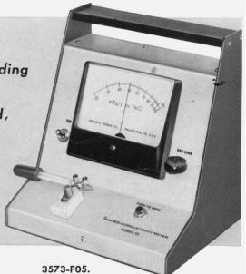
BIO-CONDUCTIVITY METER, Thomas Model 32. For rapid estimation of chloride level in sweat\* for presumptive diagnosis of cystic fibrosis. Range, 20-100 milliequivalents per liter NaCl. Test requires only 30 microliter sample, a fraction of a drop. Meter is battery-operated, lightweight and compact for bedside measurements. Readings are corrected automatically to 25°C.
