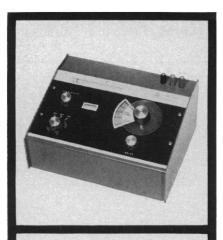
a new easy to use direct reading laboratory conductivity bridge
