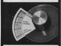
The YSI Model 31 Conductivity Bridge is brand new and specifically designed for laboratory use. Measure conductivity and resistivity with convenience, speed, and accuracy at 60 cycles or 1 kc. Use it over the entire range of electrolytic conductance from demineralized water to strong acids.
