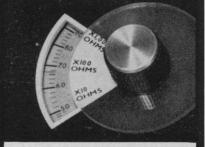
The YSI Model 31 Conductivity Bridge is brand new and specifically designed for laboratory use. Measure conductivity and resistivity with convenience, speed, and accuracy at 60 cycles or 1 kc. Use it over the entire range of electrolytic conductance from demineralized water to strong acids.
