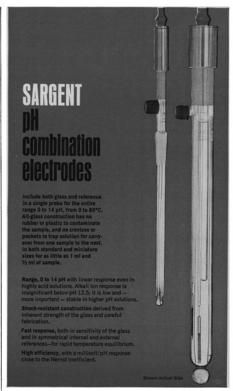
\$-30070-10 COMBINATION ELECTRODE - 0 to 14 pH, Miniature, Sargent/Jena. pH range, 0-14; temperature, 0-80°C; total length, 6 inches; stem diameter, 5mm; immersion depth, 10 to 78 mm; cap length, 1/8 inch; cap diameter, 8 mm.
