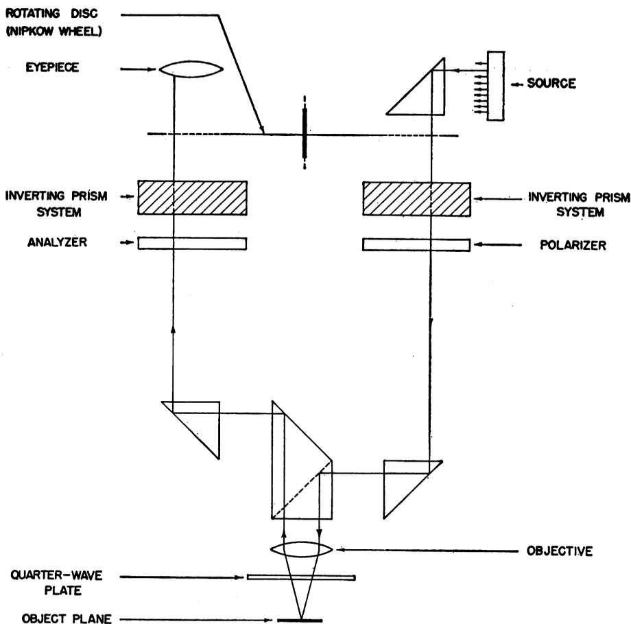
Fig. 1. Schematic diagram of microscope, tracing a single ray from light source to eyepiece and ignoring the effects of the inverting prism systems.
