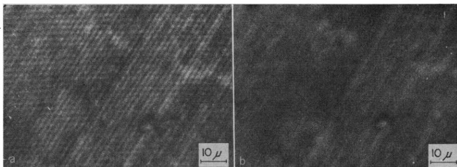
Fig. 2. Two photographs of the same portion of a reflecting replica grating ( $1.9 \mu$  per line) covered by a sheet of transparent plastic and immersed in 0.65-percent saline: with the rotating disc in the microscope (a) and with the disc removed (b).
