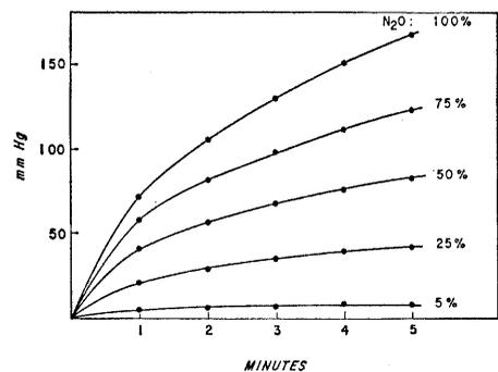
Fig. 1. Pressure within the sealed silicone rubber tube for varying concentrations of N<sub>2</sub>O in O<sub>2</sub>, plotted against time.
