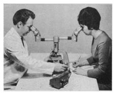
Two persons can simultaneously observe and discuss the same microscopic image at all magnifications. This microscope is equipped with two inclined binocular or monocular heads. Each viewer can focus independently. A built-in pointer can be directed to any area.
