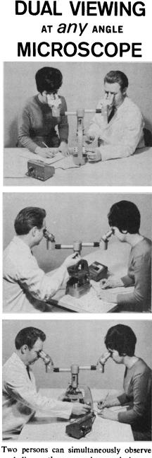
I wo persons can simultaneously observe and discuss the same microscopic image at all magnifications. This microscope is equipped with two inclined binocular or monocular heads. Each viewer can focus independently. A built-in pointer can be directed to any area.
