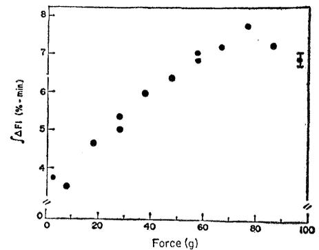
Fig. 3. Relative energy utilization in the single twitch as a function of the force developed during the contraction of toad sartorius at  $11^\circ\text{C}$  with an initial load of 2.0g; all other loads are after-loaded. Four cycles were recorded for the isometric twitch; the bar shows the spread of the data. Two cycles were recorded for the minimally loaded isotonic condition; the  $f\Delta FI$  was virtually identical for these two cycles.
