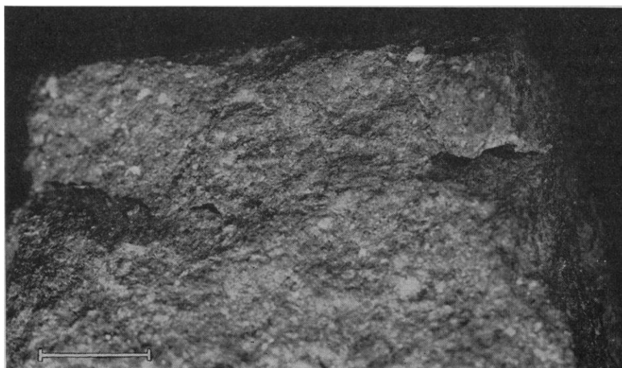
Fig. 2. A large, joint-like opening in the Farmington meteorite. The two cavities shown are roughly coplanar but are not linked by any kind of fracture or vein. Scale bar, 1.0 cm.
