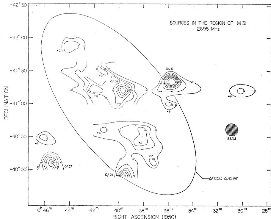
Fig. 1. Contours of constant antenna temperature at 2680 Mhz in the region of M31. Contours are labeled in degrees Kelvin.
