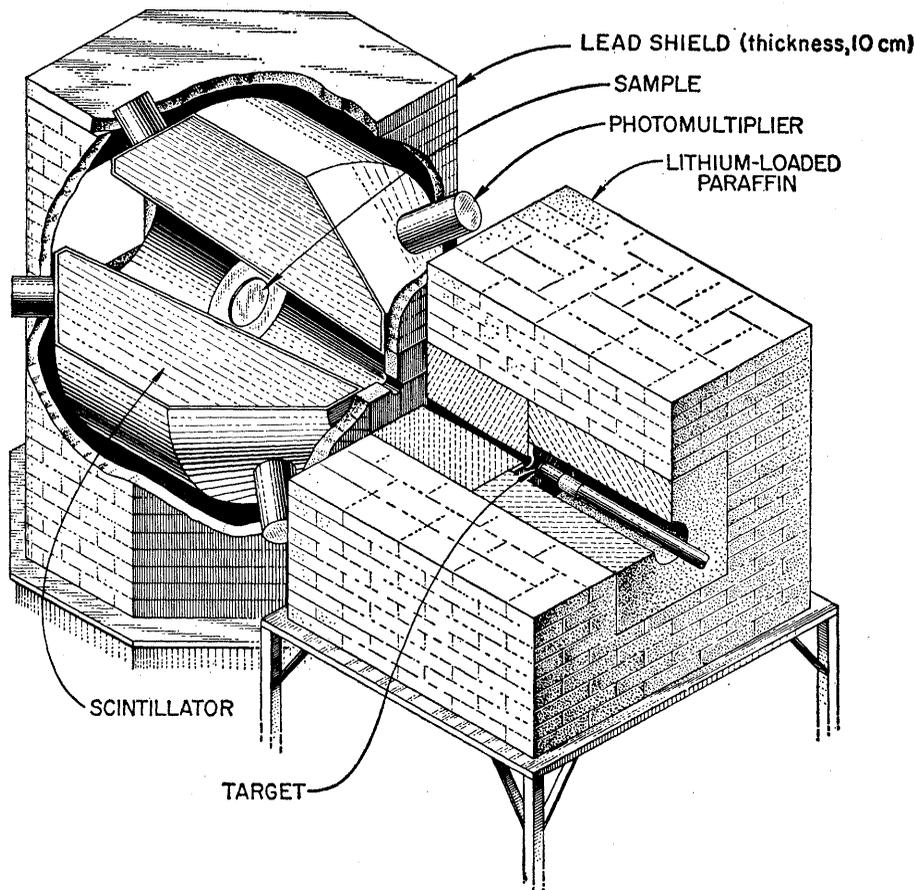
Fig. 3. Cutaway view of a large liquid scintillation detector used for neutron-capture cross section measurements. Neutrons are produced in the target by way of the  $^7\text{Li}(p, n)^7\text{Be}$  reaction. After collimation they pass through a hole in the scintillator. Those captured in the sample produce gamma rays which are detected by the scintillator. Energies of the captured neutrons are measured by measuring the time of flight from the target to the sample.
