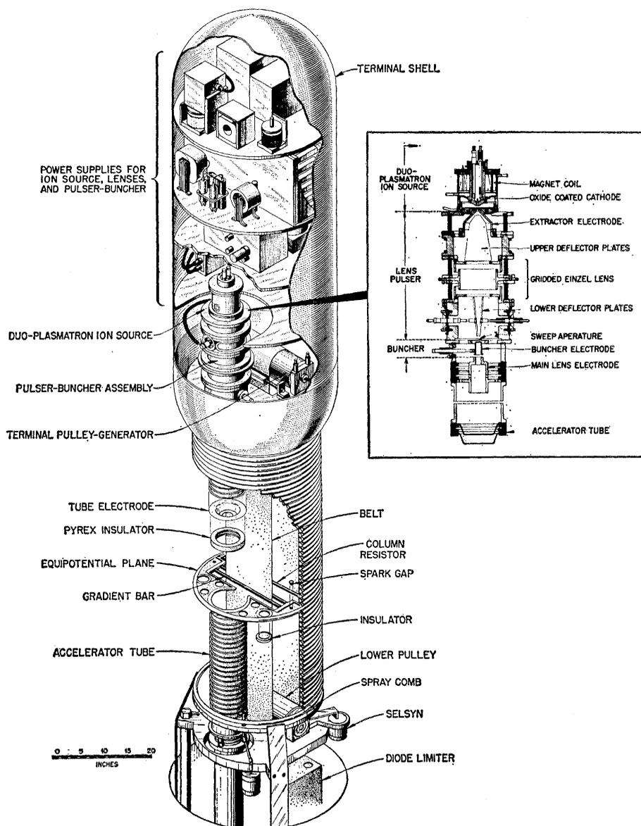
Fig. 4. Cutaway view of the Oak Ridge 3-megavolt Van de Graaff accelerator. Protons from the high-current ion sources are swept sinusoidally in an electric field across an aperture to produce short ( $\sim 10^{-8}$ -second) bursts of ions. Next the ions are "bunched" by slight deceleration of the leading edge of the pulse and acceleration of the trailing edge. This causes the pulse to be "squeezed" to  $\sim 10^{-9}$  second, the time it takes light to travel about 0.3 meter.
