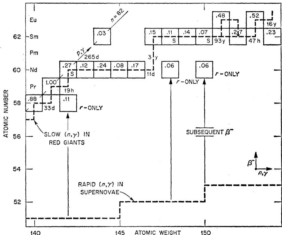
Fig. 10 (right). The s-process path near samarium. While neodymium, like tin, has one isotope produced by the s-process only, samarium has two ( $^{148}\text{Sm}$  and  $^{150}\text{Sm}$ ), and thus provided a critical test of the s-process theory.
