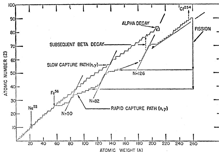
Fig. 2. The paths of the neutron-capture chains produced in the slow (s) and rapid (r) processes as proposed by Burbidge, Burbidge, Fowler, and Hoyle (8). The s-process path follows the stable isotopes; the r-process involves rapid, multiple neutron capture, later followed by beta decay.
