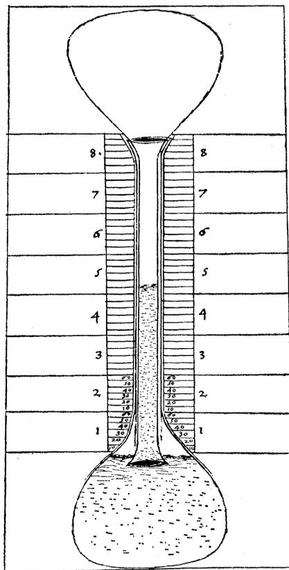
First known drawing of a thermometer, which appears in Bartolomeo Telioux's manuscript. Although Telioux was evidently not the inventor, the date of 1611 on the manuscript establishes a latest-possible date for the invention. [From *A History of the Thermometer and Its Uses in Meteorology*]
