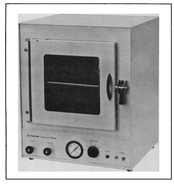
And if this isn't enough, the new Model 48 can be operated under vacuums down to 30" Hg, responds to temperature changes of  $\pm 1.0^{\circ}$  over a range of 40°C to 200°C. You can use this compact unit efficiently as a vacuum-drying oven; as a controlled-atmosphere or ordinary air-filled chamber for static drying; and as a purged-atmosphere chamber.
