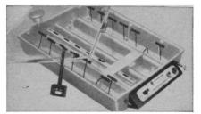
**EA-1 Electrophoresis Chamber** High impact polystyrene; water cooling jacket. Domed see-through lid. Safety interlock. Platinum electrodes run entire chamber length. Polarity reversing switch. Simple, accurate method of attaching sample strip with flexible holders in integral part of chamber unit.
