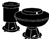
Clinical and Chemical Centrifuges Max. Speed — 8800 rpm Max. Gravity — 5550 g Max. Volume — 6 x 50 ml Versatile bench unit. Chemical model affords continuous batch separation.
