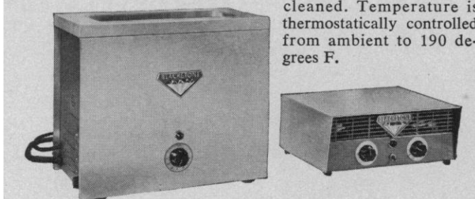
3. Blackstone U-20 Cell Disrupter. A highly flexible unit designed for routine continuous or batch processing of cell suspensions, chemicals and solutions common to research in biochemistry, cytology, microbiology and related fields. Laboratory tests show that employing a 70 ml. volume of a 20% suspension of Escherichia coli, 98% disruption was achieved in 12 minutes with no loss of activity in enzyme Beta Galactosidase. 0 to 100% power control for complete processing flexibility.
