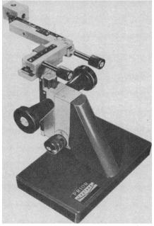
Offering resolutions of 0.0001" in the vertical plane and 0.004" in the two horizontal planes, the Micromanipulator has both coarse and vernier controls in all directions. Available accessories include Ball & Socket Joints and Adjustable Needle Holders.
