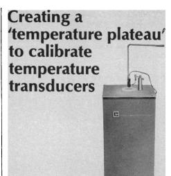
The L&N 8411 Fixed Temperature Standard consists of a vertical electric furnace and a cell containing a pure metal sample. It's virtually infallible in providing a known, fixed-reference temperature (such as the zinc-point) for calibrating resistance thermometers or thermocouples. Here's why.
