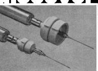
. . Swinnex® Disposable Filter Units for sterilizing or ultracleaning small volumes of liquids dispensed from a hypodermic syringe such as ophthalmic solutions, radioactive tracers and allergenic extracts. Preassembled with a sterile 0.45 or a 0.22 micron Millipore filter in place. they require no preparation before use. Write for a copy of Data Sheet SW-1325. Millipore Corporation, Bedford, Massachusetts 01730.
