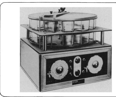
This is the Shandon-Elliott 23-station automatic slide staining machine. With it you are assured an extremely high degree of reproducibility when preparing Pap stains, blood films, bone marrow spreads and tissue sections. It is equally well suited for routine slide staining or where absolute quality from slide to slide is required. Automatic slide staining improves the performance of your lab staff by releasing skilled technicians to do other important work.
