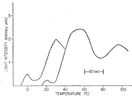
Fig. 6. This schematic glow curve gives the intensity of the emitted light as a function of the temperature as the sample is heated at the rate of  $20^{\circ}\text{C}$  per minute. The solid line is the background. The dotted line gives the signal due to illumination at  $-70^{\circ}\text{C}$ .
