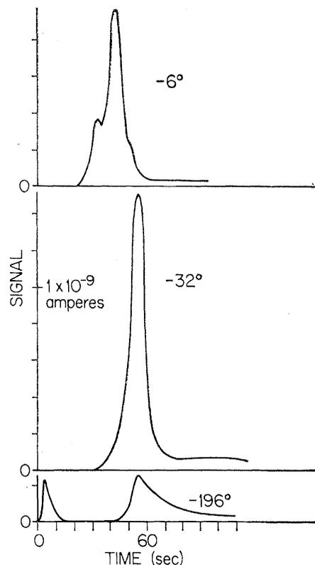
Fig. 7. Fast glow curves made with the copper plug showing the intensity of the emitted light as a function of the time of heating. The temperature of the sample at the time of illumination is shown.
