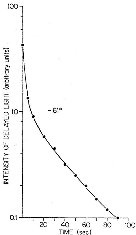
Fig. 2. Log intensity of the delayed light as a function of the time of illumination. The nonexponential nature of this decay may be due to the use of thick (6.5 mm) samples. Use of the aluminum bar for cooling made it necessary to use the thick samples.
