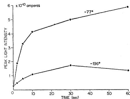
Fig. 3. Peak light intensity as a function of the time of illumination. The shape of the light signal was determined by the electrical circuits, time constant of 9 seconds. The temperature of the sample was raised from  $-190^{\circ}\text{C}$  to  $+95^{\circ}\text{C}$  by immersing it in a pan of hot water.
