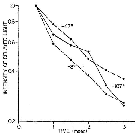
Fig. 1. Log intensity of the delayed light as a function of time. Time is measured from the instant that the second shutter starts to open. The delayed light signals have been normalized to unity at  $\frac{1}{2}$  msec.
