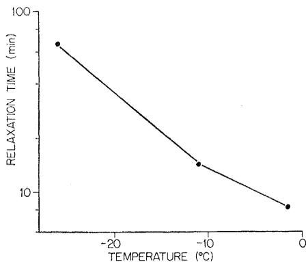
Fig. 5. The relaxation time (time to decrease to 37 percent) is plotted as a function of the temperature. The points were calculated on the assumption that the decay was exponential.
