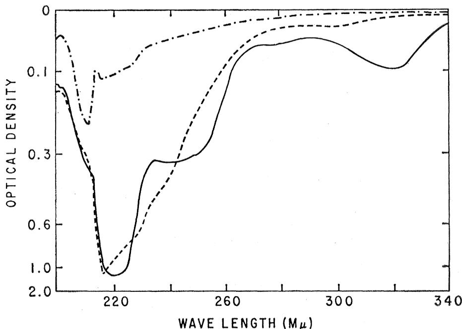
Fig. 2. Ultraviolet absorption spectra of PCNB and its degradation product (pentachloroaniline). Ether solutions contained 10  $\mu\text{g}$  of either compound per milliliter. Ether, — · — · —; PCNB, — — —; degradation product, — — —.
