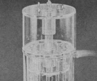
The Poly Analyt is a truly compact and convenient-to-use analytical apparatus that offers unmatched flexibility, efficiency and economy of operation. Gives complete electrophoresis separation in 30 to 45 minutes.
