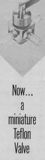
Here's a small  $(\chi_{6}" \times 1")$  valve constructed of Teflon and Kel-F in a sturdy metal housing. It is gastight and essentially inert, and is ideal for controlling gases or liquids in a miniature piping system. Available with two, three, or four ports, and a variety of standard luer fittings.
