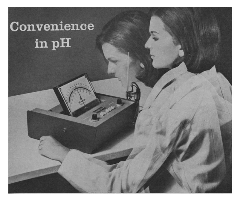
No need to squint or squirm. New Photovolt pH Meter 111 has unique tilting meter for precise glare-free reading and pushbutton controls for convenient operation.
