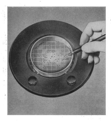
Bacterial colonies can be recorded quickly and accurately in a *single* probing action with the Bactronic Colony Counter, which marks as it counts automatically in open and closed petri dishes. An electronic probepicks up radio impulses on contact with any agar medium, actuates the counting mechanism, and leaves an identifying puncture in the agar. If puncturing is undesirable, a plug-in marking pen or grease pencil can be used to mark the back of the plate as it counts. A
