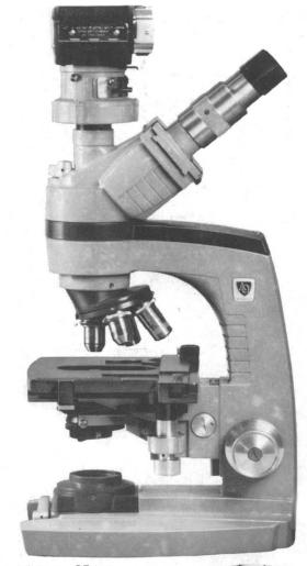
More plusses: 35mm, Polaroid® or 4 x 5 photography; an auxiliary viewing screen; minimum slide breakage because the objective nosepiece floats if contact is made with slide; minimum maintenance throughout.
