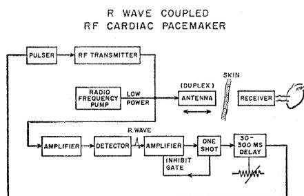
Fig. 1. Schematic diagram of the equipment.
