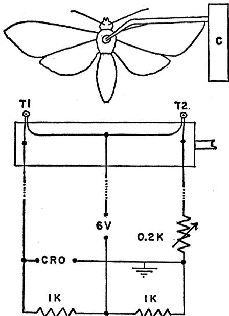
Fig. 1. Diagram of differential anemometer. C, phono-pickup bearing stylus to which moth is attached; T1 and T2, bead thermistors attached to plastic strip and placed in wake of flying insect; and CRO, cathode ray oscilloscope. Components of bridge circuit as indicated; 1K equals 1000 ohms.
