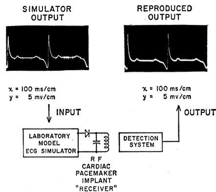
Fig. 2. Results with the output (up to 10 mv) of a cardiac-voltage simulator applied to the electrode leads.
