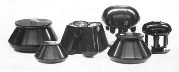
Derating of ultracentrifuge rotors is a necessity brought about by the development of progressive metal fatigue as a consequence of long-continued or repeated stressing under extremely high centrifugal forces. This is usually expressed as successive limitations in permissible top speeds.
