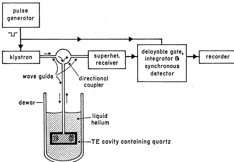
Fig. 1. Block diagram of "single-ended" ultrasonic pulse-echo apparatus. Sound pulses are generated and detected simultaneously at both ends of a quartz rod which completely fills a rectangular  $\text{TE}_{215}$  cavity. For any given echo, synchronous detector compares output (of superheterodyne receiver) containing noise-plus-signal with noise only.
