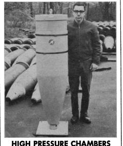
Project Plowshare: At Benthos we are converting weapons into laboratory instruments. High strength steel 16" U.S. Naval gun shells are being made into inexpensive hydrostatic pressure testing chambers. Inside is 9.4" diameter, 46" long. Rating is 10,000 psi. Cost is \$1400. Join the Plowshare Program. Call or write Benthos today.
