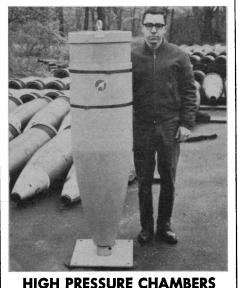
Project Plowshare: At Benthos we are converting weapons into laboratory instruments. High strength steel 16" U.S. Naval gun shells are being made into inexpensive hydrostatic pressure testing chambers. Inside is 9.4" diameter, 46" long. Rating is 10,000 psi. Cost is \$1400. Join the Plowshare Program. Call or write Benthos today.
