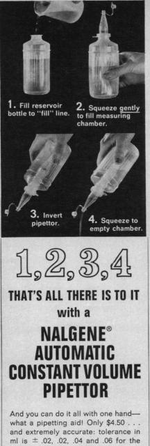
ml is  $\pm$  .02, .02, .04 and .06 for the 1, 2, 3 and 5 ml sizes, respectively. Use several for procedures requiring repeated dispensing of different
