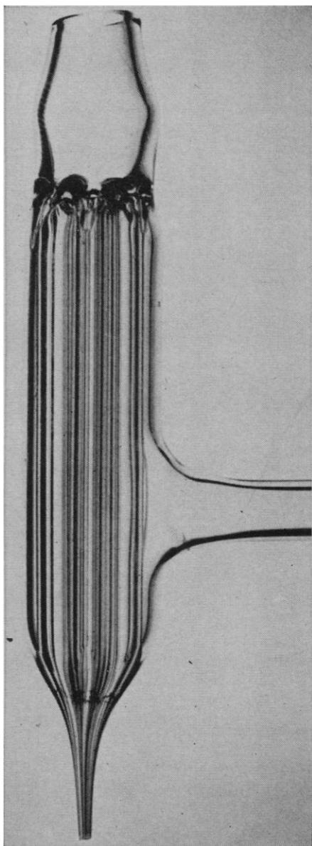
Fig. 1. Multicapillary mixer.
