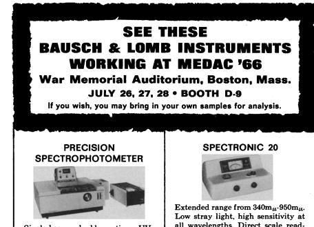
Single-beam, double-grating. UVvisible range:  $190m_{\mu}$ -700m<sub> $\mu$ </sub>. Large sample compartment (6" x 6" x  $8\frac{1}{16}$ "). Choice of collimating or focusing optics. Wavelength accuracy -...5A. Wavelength graduations-.2m<sub> $\mu$ </sub>. Combination light source. Constant bandpass-2A, 5A and 20A.
