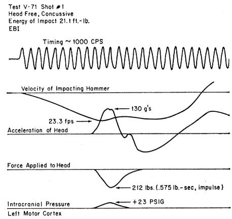
Fig. 1. Oscillographic record of physical measurements during impact; traces for velocity, acceleration, force, and intracranial pressure with a 1000-cy/sec time trace are displayed.
