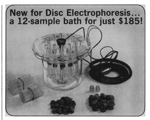
The new Canalco Model 66 Bath Assembly now lets you run twelve samples at a time with unmatched convenience and economy. Based on a bath design proven in hundreds of laboratories all over the world, the Model 66
