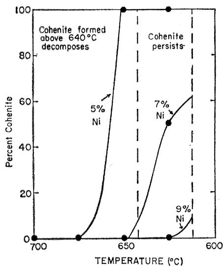
Fig. 4. Cumulative percentage of cohenite formed during cooling plotted against temperature for 3 meteorite compositions, each containing 0.3 percent carbon. Ordinate represents percentage of cohenite present with respect to the total cohenite which would form if all the carbon present were in the form of cohenite. The vertical dashed line at right is 610°, below which cohenite does not form.
