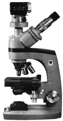
More plusses: 35mm, Polaroid® or 4 x 5 photography; an auxiliary viewing screen; minimum slide breakage because the objective nosepiece floats if contact is made with slide; minimum maintenance throughout.
