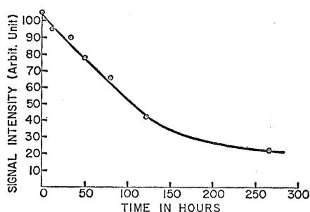
Fig. 2. Decay curve of methyl radicals at room temperature.
