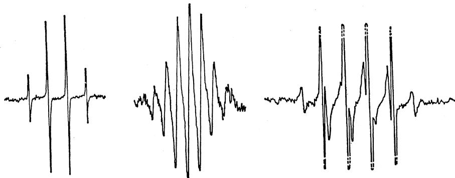
Fig. 1. ESR absorption derivative spectra of methyl (left) and deuteromethyl (center) and C<sup>13</sup>-methyl (right) radicals at room temperature.
