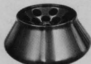
A-90 ALUMINUM 16 x 55 ml — 25,000 rpm. 90,100 g
