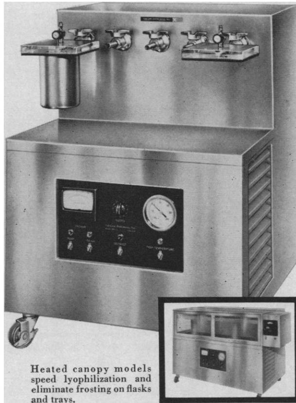
Heated canopy models speed lyophilization and eliminate frosting on flasks and trays.
