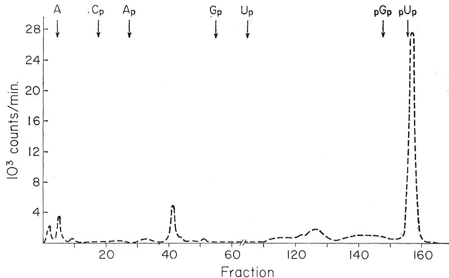
Fig. 3. Column chromatography (Dowex-1) of an alkaline digest of  $S^{35}$ -labeled sRNA. Elution positions of the nucleotides are indicated by arrows. The first two peaks represent methionine and cystine (6 percent of total radioactivity) whereas the major peak accounts for 50 percent of the total radioactivity. The remaining components have not been identified.
