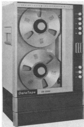
VR-3300 Magnetic Tape Recorder/Reproducer
