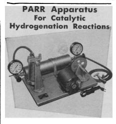
Numerous reactions with hydrogen at pressures up to 5 atm. (60 psig.) can be performed in this convenient shaker apparatus using either 250 or 500 ml. pressure-tested glass bottles.
