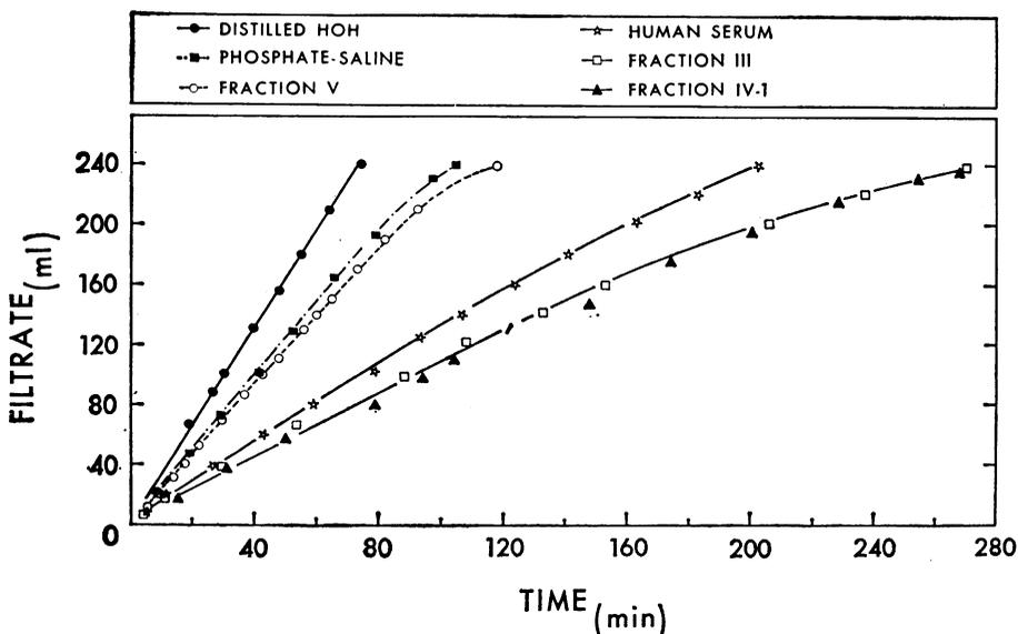
Fig. 2. Filtration rates of various solutions through the same Diaplex membrane. Filtration order: fraction V, fraction IV-1, human serum, fraction III, phosphate-saline buffer, and distilled water. Pressure used was 6.8 atm and the effective surface area was 20.2 cm<sup>2</sup>.
