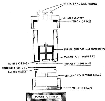
Fig. 1. Vertical cross section of the Diaplex membrane filtration apparatus.
