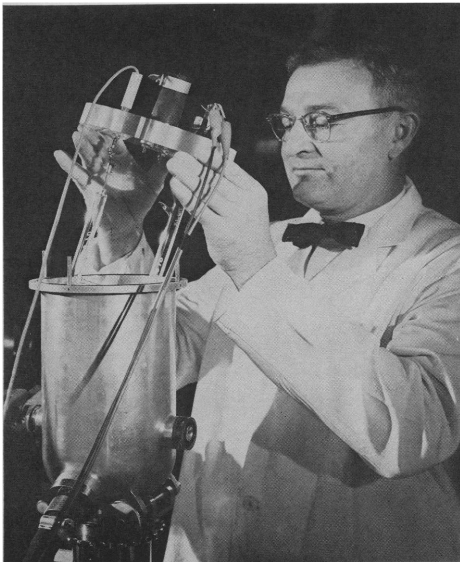
Fig. 2. A National Bureau of Standards scientist inserts a krypton-86 lamp into its liquid-nitrogen bath. The wavelength of the orange-red light emitted by the lamp has been adopted as the international standard of length. The lamp is operated at liquid-nitrogen temperatures to increase the stability of the standard wavelength.
