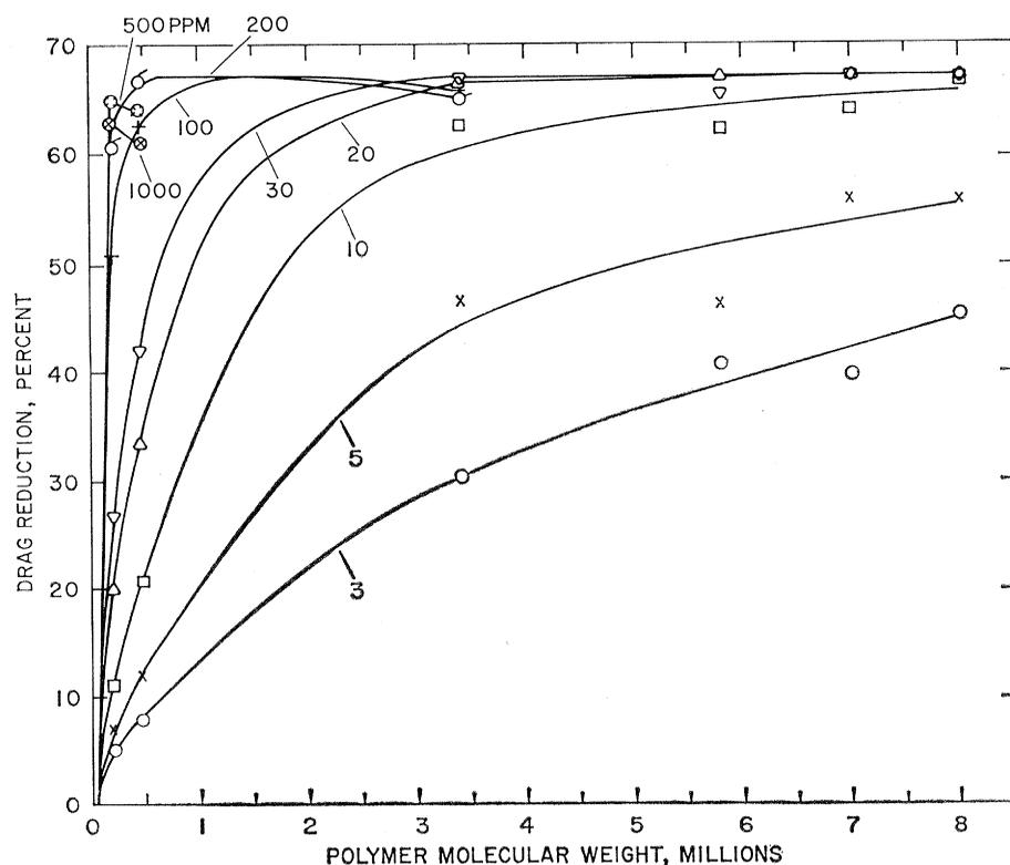
Fig. 3. Chart for estimating molecular weight of polysaccharide, based on test data on poly(ethylene oxide).
