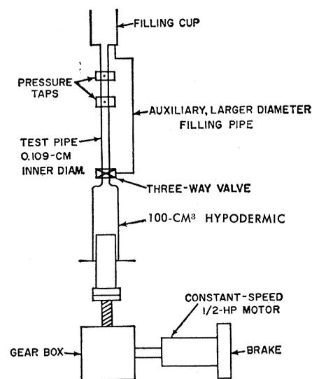
Fig. 1. Diagram of apparatus for measuring pressure losses by turbulent friction, caused by flow of algal cultures through a test pipe.
