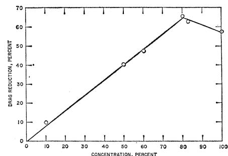
Fig. 2. Effect of dilution of culture of *Anabaena flos-aquae* with distilled water on observed reduction of friction.
