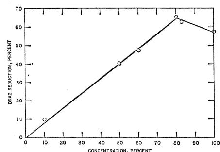
Fig. 2. Effect of dilution of culture of *Anabaena flos-aquae* with distilled water on observed reduction of friction.
