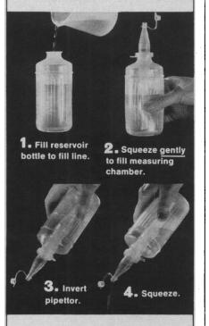
Use several for procedures requiring repeated dispensing of different reagents. Unbreakable ... resists most chemicals. Disassembles in seconds for cleaning and refilling. All units have 8-oz. polyethylene reservoir bottle with choice of 1, 2, 3, or 5 ml polypropylene measuring chamber. Price, \$4.50 each. May be assorted with other Nalgene Labware for maximum discount. Ask your lab supply dealer, or write Dept. 21201, The Nalge Co., Inc., 75 Panorama Creek Drive, Rochester, New York 14625.
